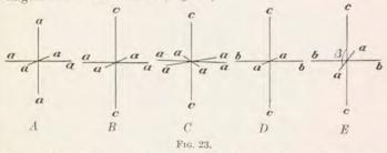
Axes of CRYSTAL SYSTEMS.—A. Isometric; B. Tetragonal (the vertical axis c-c being longer or shorter than the horizontal axes); C. Hexagonal; D. Orthorhombic; E. Monoclinic (there being an oblique angle  $\beta$ , between the a and c axes).
